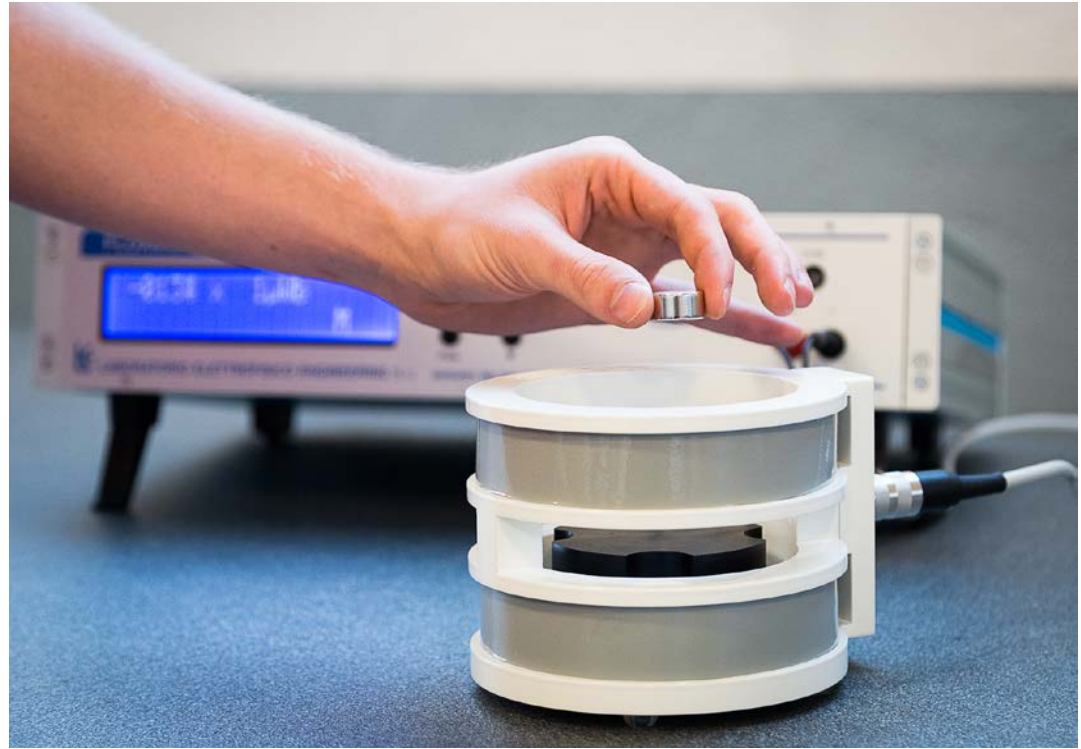
The measure of magnetic moment with Helmholtz coils (in the pictures, connected to a fluxmeter)
